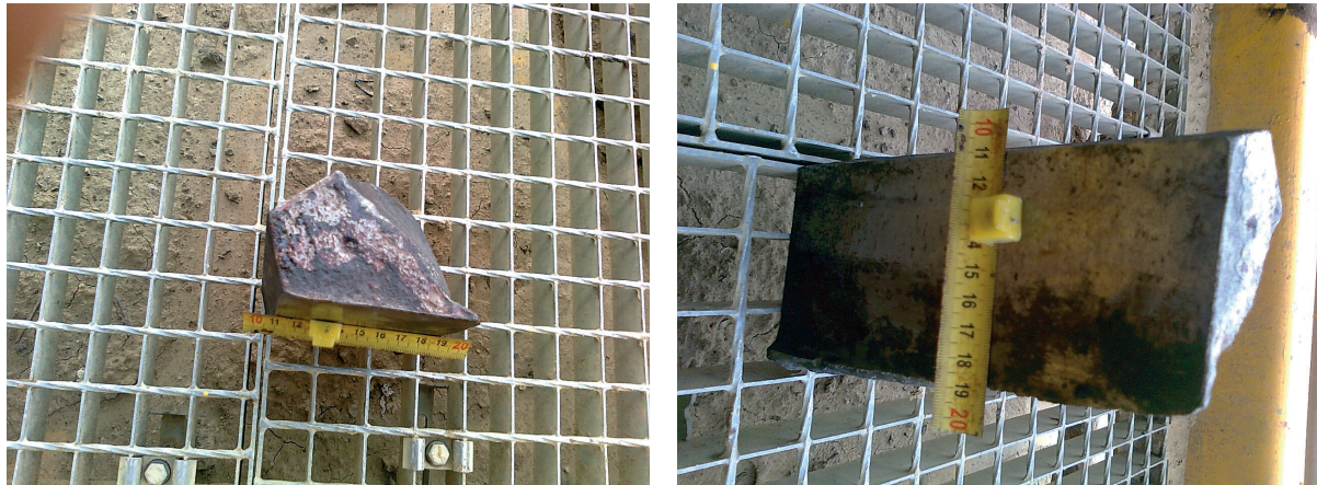
Figure 3 Appearance of the broken tooth and its dimensions
